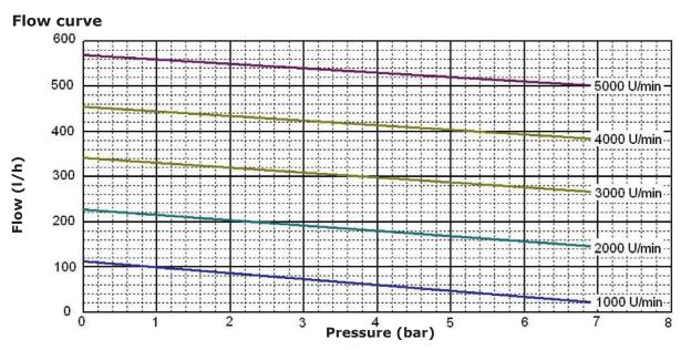
Performance curve based on: medium water, temperature 20°C, viscosity 1 cP, bypass closed
